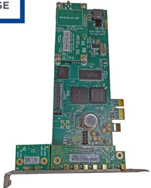
**Safran's CDM-7 clock distribution and timing reference module is a PCIe card that provides 10MHz and 1PPS signals for up to seven devices that need precise synchronization.**
